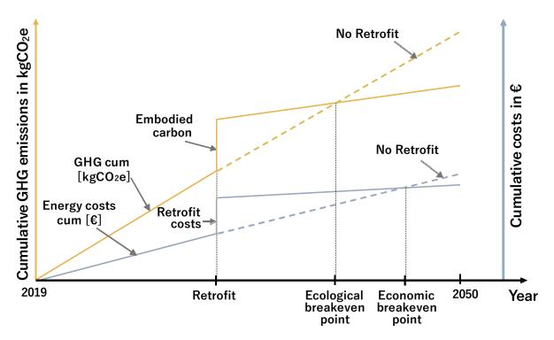
**Figure 8:** Cumulative GHG emissions, energy costs, and breakeven points of retrofit measures including embodied carbon and retrofit costs (in kg/CO<sub>2</sub>e and EUR)
