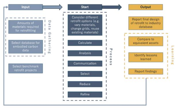
Figure 17: Process map for implementation of embodied carbon calculations<sup>63</sup>
